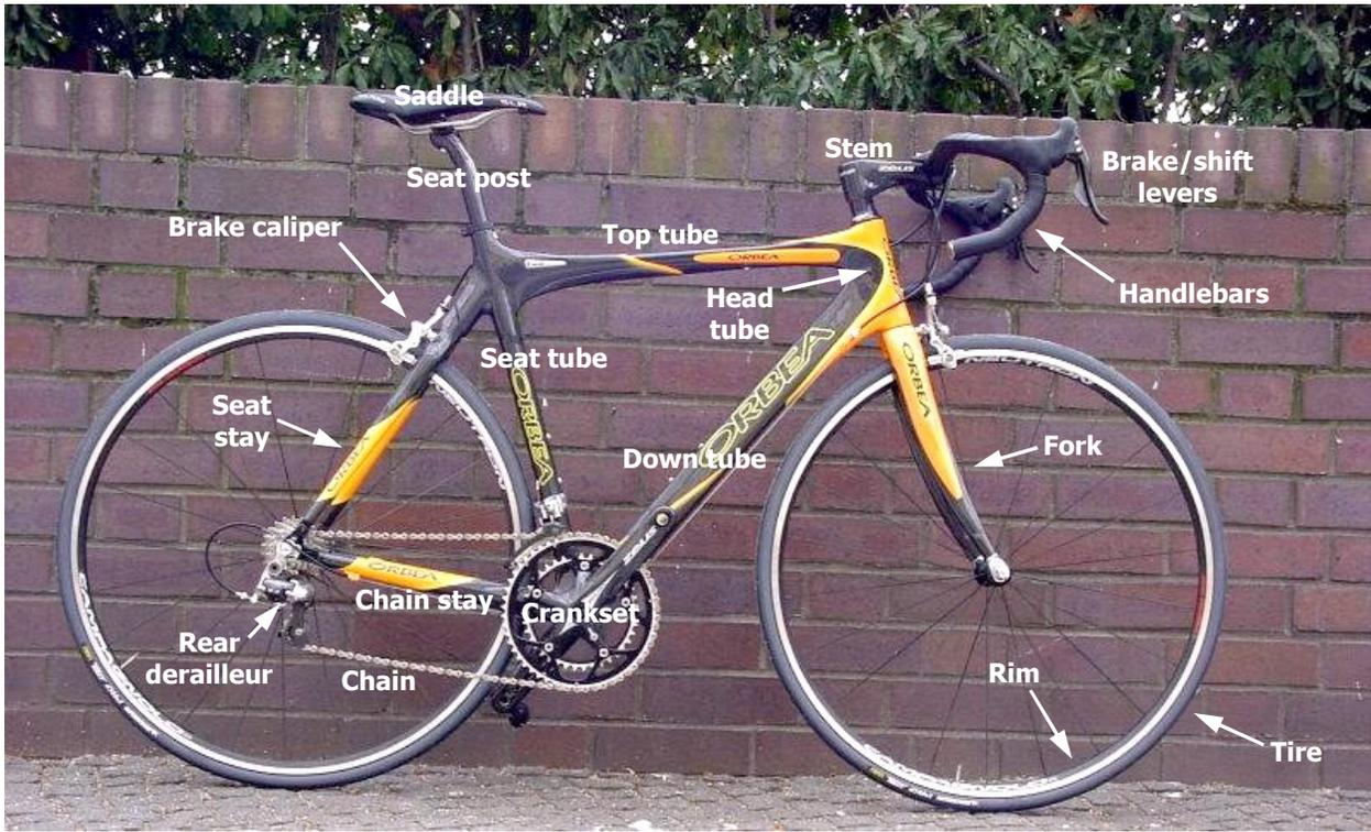
Components of an 18-speed, carbon-fiber framed racing bicycle (pedals omitted).
